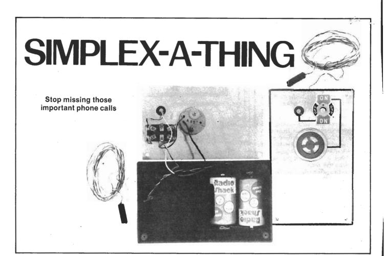
YOU WON'T MISS any more phone calls when out of hearing range of your telephone, if you add this simple remote signalling unit which alerts you to incoming calls by means of either a buzzer or blinker light. The unit is self powered for easy placement in any room in your home, or even outdoors where there are no AC outlets.
